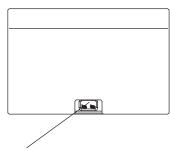
Recessed connector pockets for safety of cables and connectors
