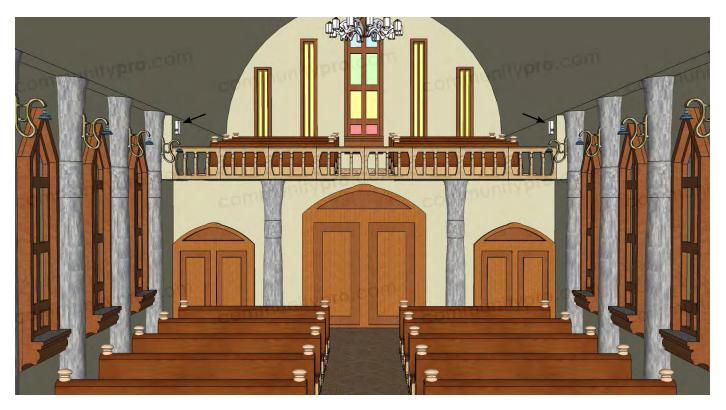
The above view shows the two ENT203s that cover the balcony, one on either side. Below is a 3D rendering depicting highly uniform coverage throughout the front, sides, and rear.
